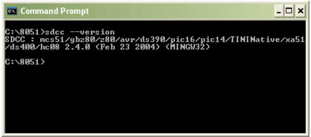
Figure 1. Verifying the Correct Installation of the SDCC by Performing a Version Check
